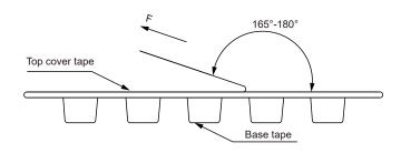
The peel force of top cover tape shall be between 0.14 to 0.78 N
