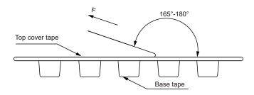
The peel force of top cover tape shall be between 0.1 to 1.0 N
