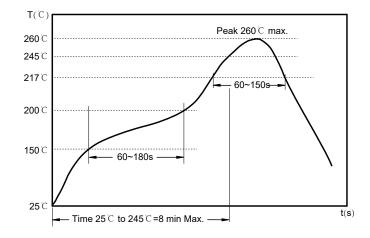
Preheat condition: 150 ~200 °C / 60~180 sec. Allowed time above 217 °C : 60~150 sec. Max temperature: 260 °C. Max time at max temperature: 10 sec. Allowed Reflow time: 3x max.
