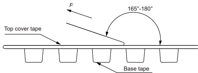
The peel force of top cover tape shall be between 0.10 to 1.17 N
