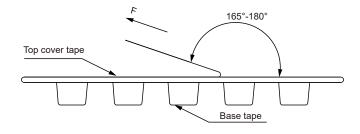
The peel force of top cover tape shall be between 0.10 to  $1.17~\mathrm{N}$
