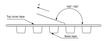
The peel force of top cover tape shall be between 0.20 to 1.17  $\mbox{N}$
