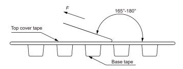
The peel force of top cover tape shall be between 0.10 to 1.17 N
