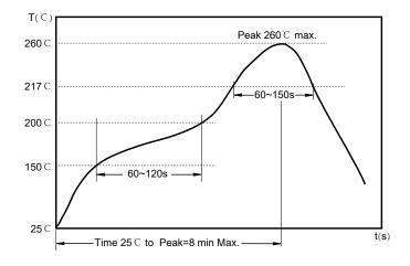
Preheat condition:  $150 \sim 200^{\circ}$ C /  $60 \sim 120$  sec. Allowed time above  $217^{\circ}$ C :  $60 \sim 150$  sec. Max temperature:  $260^{\circ}$ C. Allowed Reflow time: 3x max.
