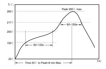
Preheat condition: 150 ~200 °C / 60~120 sec. Allowed time above 217 °C : 60~150 sec. Max temperature: 260 °C. Allowed Reflow time: 3x max.
