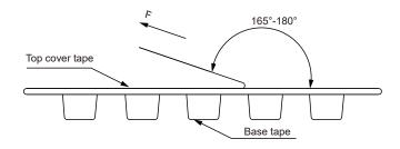
The peel force of top cover tape shall be between 0.14 to 0.58 N
