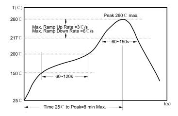
Preheat condition: 150 ~200 °C / 60~120 sec. Allowed time above 217 °C : 60~150 sec. Max temperature: 260 °C. Max time at max temperature: 10 sec. Allowed Reflow time: 2x max.
