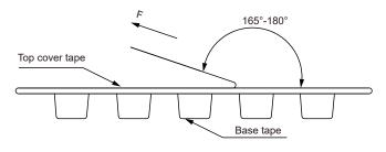
The peel force of top cover tape shall be between 0.1 to 1.3 N
