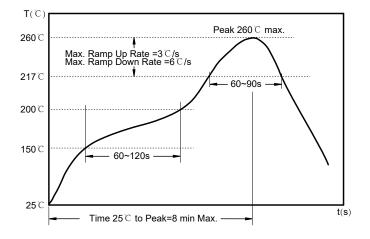
Preheat condition: 150 ~200 °C / 60~120 sec. Allowed time above 217 °C : 60~90 sec. Max temperature: 260 °C. Max time at max temperature: 10 sec. Allowed Reflow time: 2x max.
