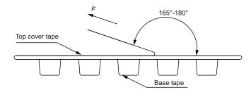
The peel force of top cover tape shall be between 0.3 to 1.17  $\mbox{N}$
