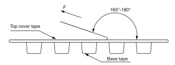
The peel force of top cover tape shall be between 0.1 to 1.17 N
